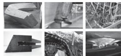
Fig. 1 top: 'Centre Pompidou Metz' (Shigeru Ban): glulam sections before milling; 5 axis milling of glulam girders; mounting of the girders on the building site; bottom: 'Hungerburgbahn' (Zaha Hadid Architects).
