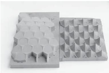
Fig 7 *3D milled mould for deep drawing*
