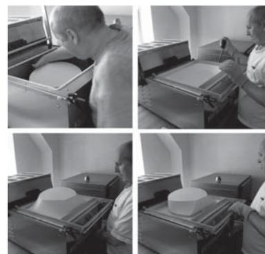
Fig. 4 Vacuum deep drawing at the model building workshop, material white polystyrene and polyurethane (mould).
