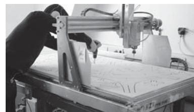
Fig. 5 3-axis portal milling machine at TU Vienna
